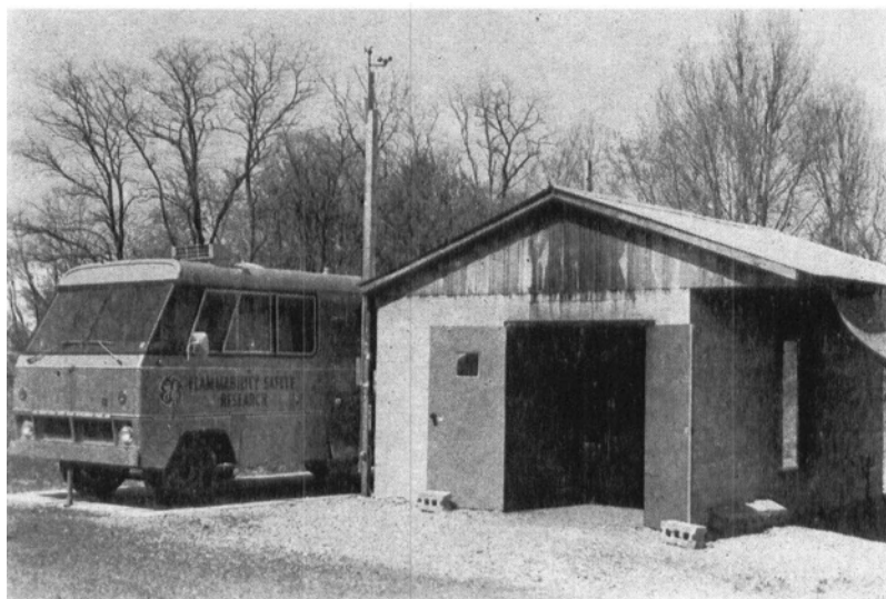
FIGURE 7 General Electric Plastics Division Fire Test Center at Mt. Vernon, Indiana. The Center includes a fire test room, center right; a mobile analytical laboratory, left; and a storage building. Since real fire behavior is sensitive to weather, a weather station is included as part of the instrumentation.
